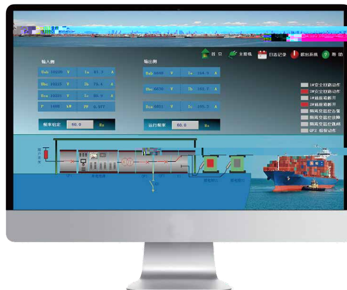
Shore Power Monitoring System
